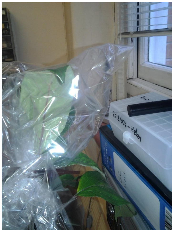
Figure 7.2. Solid phase microextraction (SPME) collection from an apple, Malus domestica , shoot in the lab at NRI.
